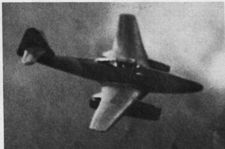
Twin-jet Me-262 has swept-back wing of irregular shape. Jet units are large and underslung. Sleek fuselage has long, pointed snout.
